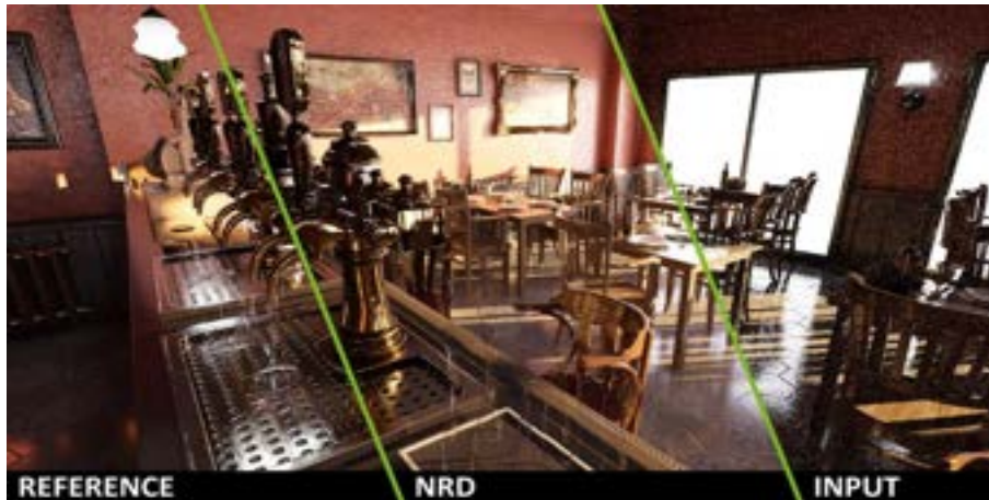
Figure 2.4.1: Example scene that illustrates the performance of NVIDIA’s real-time denoiser (NRD). On the right we can see the input image containing a severe level of noise. In the middle the reconstructed image by NRD. On the left the reference image rendered with a very high amount of samples per pixel.
