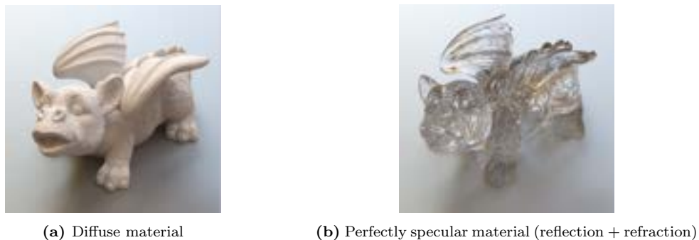
Figure 1.2.1: Example renders of the dragon model using a standard diffuse material (a) and a perfectly specular material that is reflective and refractive (b). Due to the light being uniformly reflected on the surface’s hemisphere, we observe that the diffuse material has a matte appearance. In contrast, specular highlights are visible on the perfectly specular material. Renders from [31].
