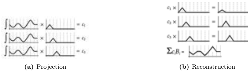
Figure 2.3.3: a: We calculate basis function coefficients c_i by integrating the product of the original function f and each basis function B_i over the full domain of f . b: We approximate the original function f by summing over each basis function B_i scaled by c_i . Figure from [13].
