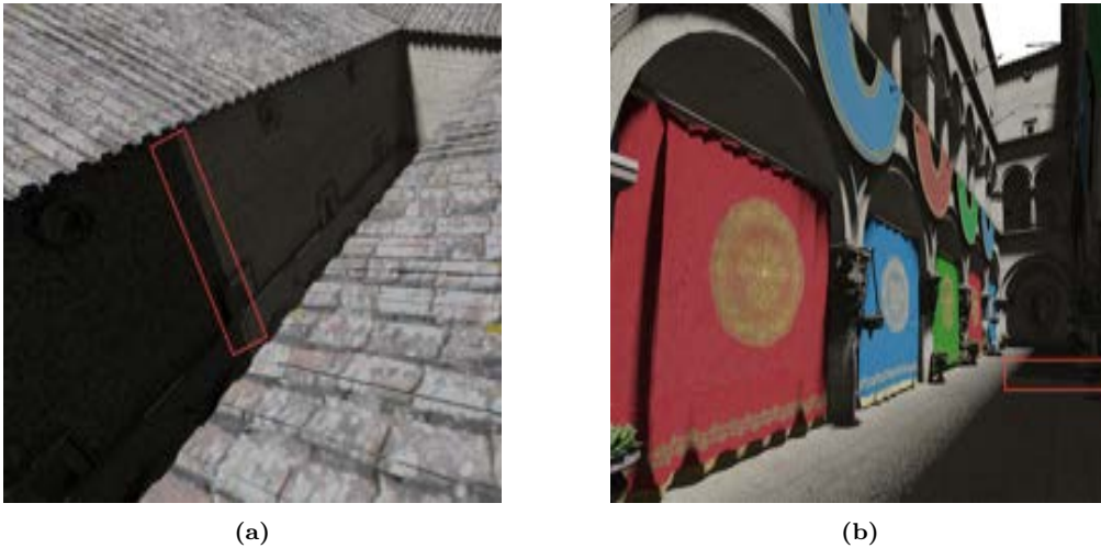
Figure 4.3.5: Dark leak artifacts appearing in renders of the Crytek Sponza scene (8 samples for direct lighting, 10 samples for indirect lighting) using the biased version of our algorithm, with a tracing range set to 0.025.
